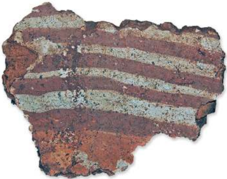
Fig. 15b: Clay mortar plaster from the walls of the Grat Be'al Gebri (DAI, Daniela Geyer)
